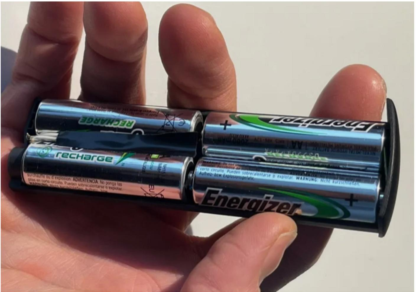
As you can see above, this is how a rebuilt battery that can be recharged by the newton should look like, you should use rechargeable cells and at the top is the thermal fuse soldered in place and to the bottom center you can see the thermistor installed and taped to the cells to monitor the temperature of the cells by the newton when recharging. The thermistor is soldered to the two terminals at the bottom of the battery tray so it can be detected by the newton hardware.
